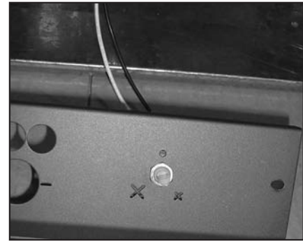
Figure 50. Install Fan Controller Nut.
